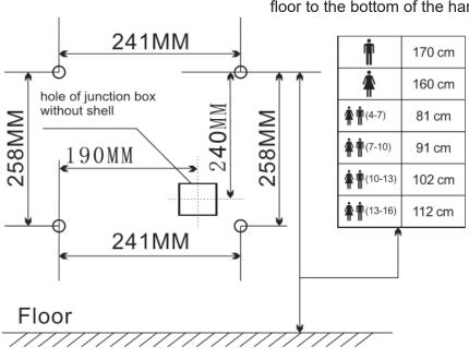
This is the mounting height from the floor to the bottom of the hand dryer.
